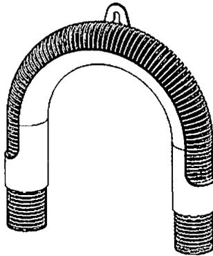
5. Attach drain hose hanger (shipped in washer tub) to drain hose.
